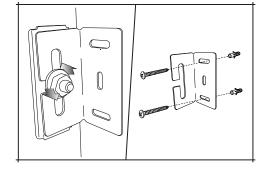
To remove the doors simply open the door and press the button at the back of both hinges.
