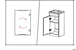
One door units will arrive with the door with the hinges attached, dissassembled from the carcass of the unit. Decide whether you want Right or Left hand opening and orientate the door accordingly. Then secure the hinges to the carcass through the predrilled pilot holes.
