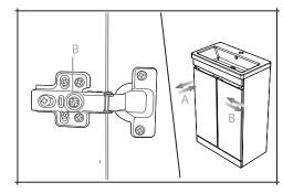
One and Two door units can be adjusted by the screws on the door hinges.
